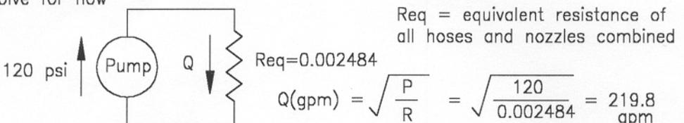
EXAMPLE 2b Calculate the flow in the individual hoses.
